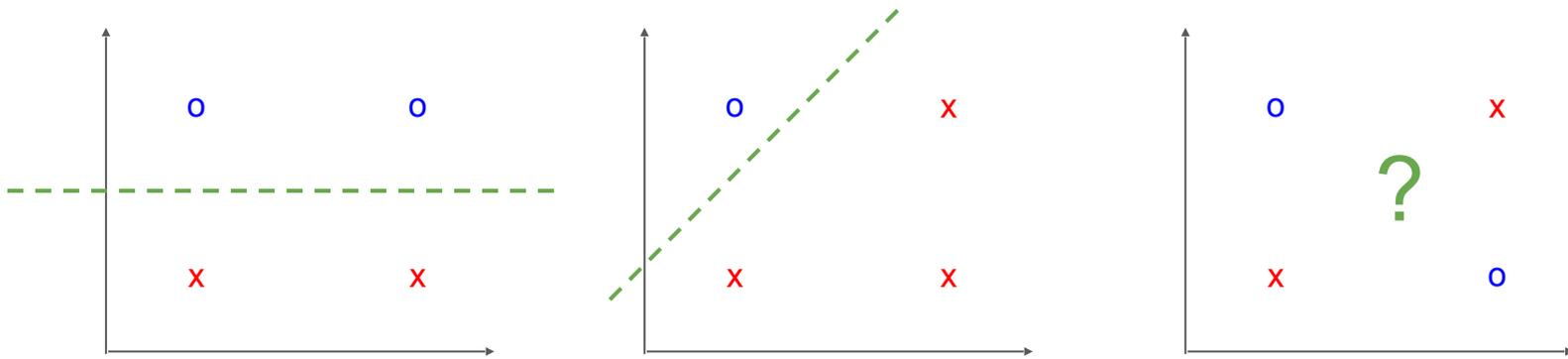
Datasets where class can be separated by a straight line (hyperplane) are called **linearly separable**.
